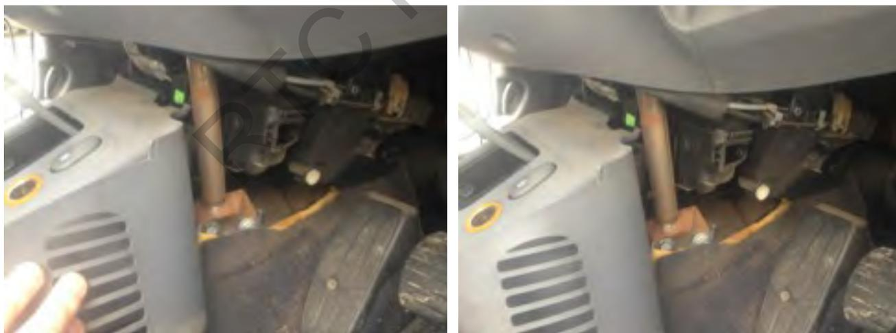
You can see the bolts holding it in place in these pictures, one option would be to unbolt or cut the post, is this a realistic option? Time frames will have to play a big part in the decision making processes along with access to this area depending on vehicle and casualty location/ orientation.
