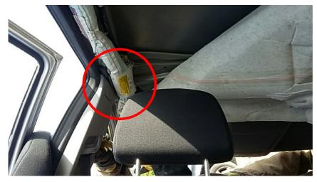
You can see in the diagrams that the inflation cylinder was in line with the Cantrail/side header rail above the B-pillar on a side resting vehicle. 'picture rotated for ease of viewing'
