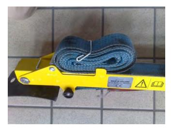
When you get to work all you need to do is just take the ratchet strap from under the sprung clip and extend and fit the StaBfast with ease, and without the need to pull the strap from the spring unit, as it will now be free with no friction on it.
